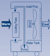
Water from an onboard tank is pumped to the top of a filterlike cooling pad. Then, a 3100 CFM fan pulls warm, environmental air over the filter and pushes out air with a cooling effect 30+ feet.
