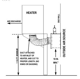
FIG. 4d Alternate Air Inlet Locations
