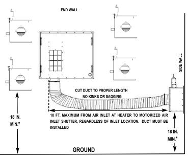
\* THE MOTORIZED AIR INLET MUST BE INSTALLED A MINIMUM OF 18 IN. ABOVE THE GROUND OR TO A HEIGHT NECESSARY TO PREVENT BLOCKAGE FROM OBSTRUCTIONS (EXAMPLES: SNOW, EXTERIOR PLANT GROWTH, ETC.)
