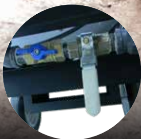
Switch between LPG and NG with push lever on DF unit
