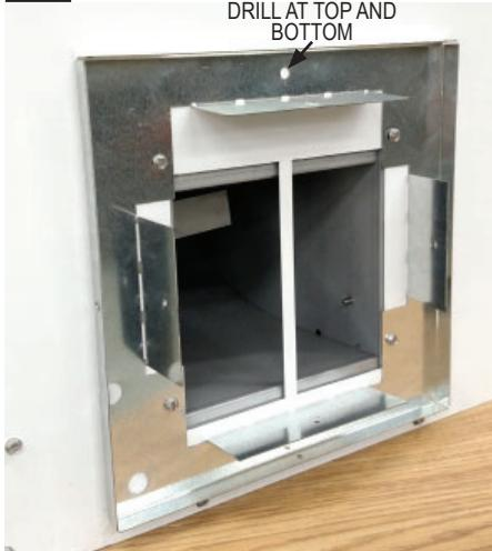
3. Position the inner duct with dampers to the four inner mounting tabs of the take off flange. See Fig. 9. Ensure the dampers of the inner duct lift and drop as shown in Fig. 10. Fasten the inner duct to the take off flange, using quantity 4 item F screws. Tighten securely.
