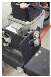
2. Position the sheet metal cover over the gas valve and slide it between the gas valve brackets.
