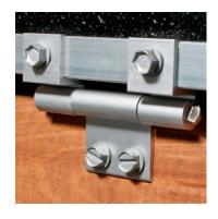
Standard heavy duty extruded aluminum hinge with stainless steel pin and wide leaf at bottom to prevent wood from splitting during installation.
