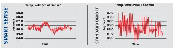
1.) Temperatures recorded in degrees Fahrenheit 2.) Test site location- Midwest Layer House (20,000 birds) 3.) Test duration- January '12 - February '13. Results- Saved 15% on fuel, 1600 gallons.
