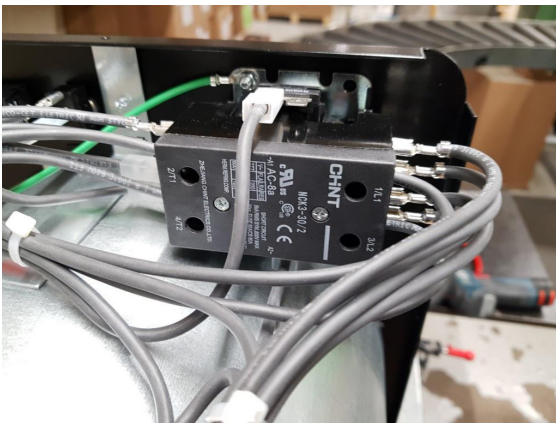
Figure 1 - Contactor Chint NCK-30 (Part# 22670)
