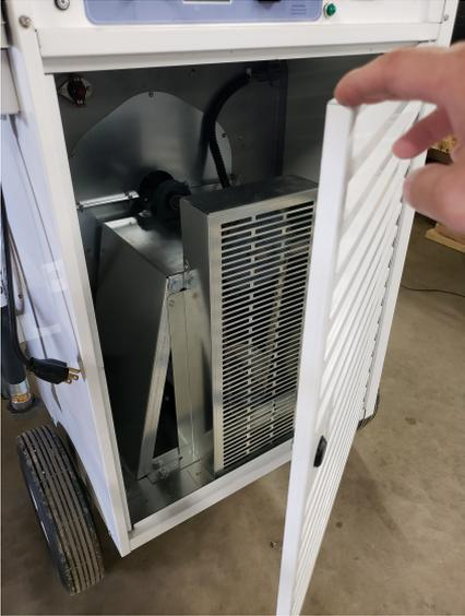
2. Locate the face plate and remove the screws and nuts to expose the connector slot on the heater. Save the screws and nuts. See Fig. 2.
