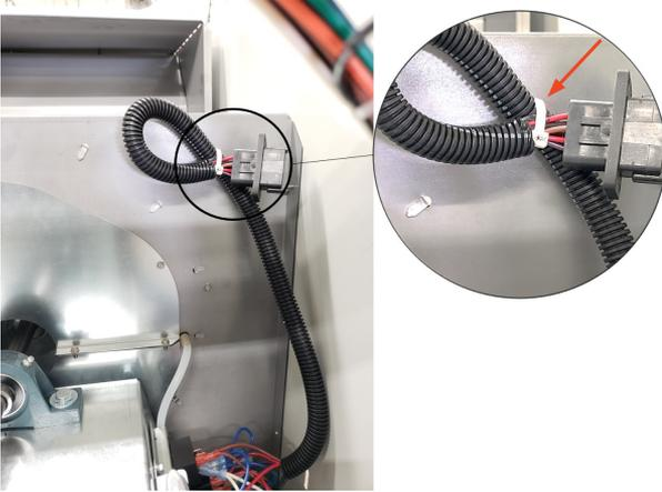
4. From inside the heater, insert the 12 pin relay harness connector through the connector slot and secure it from the outside with the screws and nuts removed earlier. See Fig. 4.
