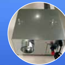
Air inlet relocated to follow heater tubes
